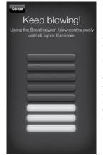
Step 3. When the screen on your mobile device reads, "Blow now," take a deep breath, and blow into your BACtrack Mobile Breathalyzer continuously until all the bars are illuminated. It should take about five seconds, and you might hear a click towards the end - that's the air pump pulling air across the sensor.
